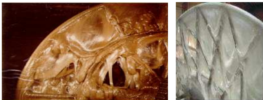
Figure 1.2.6 Thin film formation in DISCAGE ® reactor [21] .
