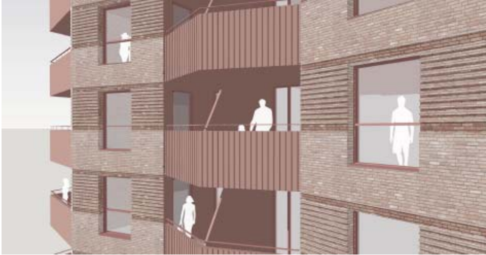
Metal balcony design and brick corbelling
