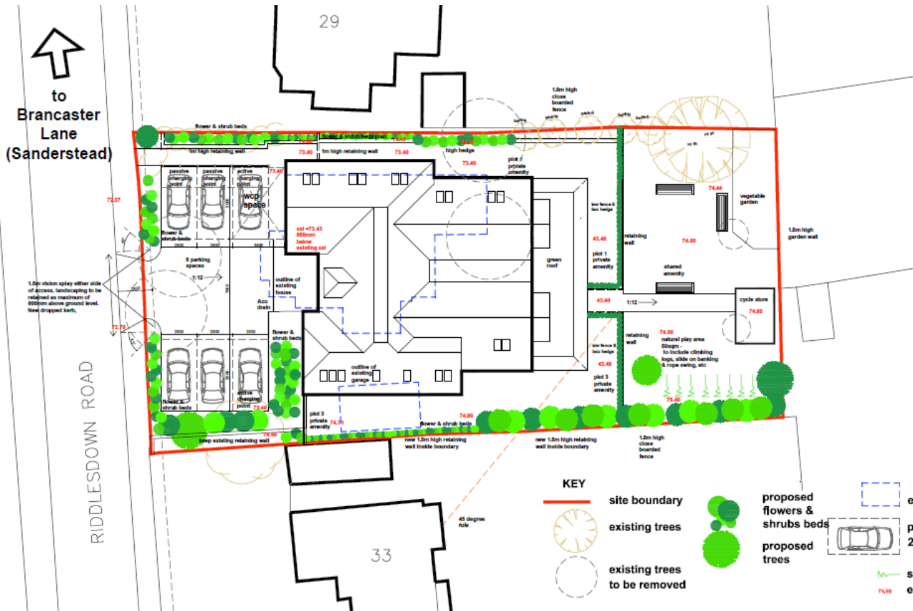
Figure 3: Ground floor plan proposed site showing proposal in relation to neighbouring properties
