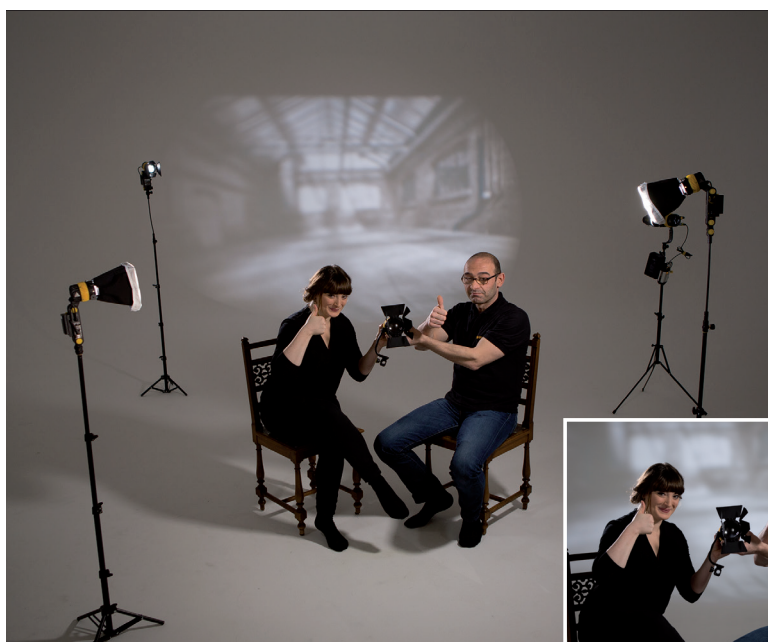
Picture shows setup with 3 DLED4 lights, background projection with DLED4 (40 W) light head plus imager.
