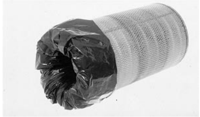
Air Intake Leak Test
