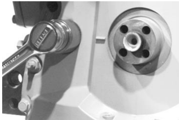
Remove Oil Pressure Regulating Valve Plug (Early Two-Valve Head Engines Only)
