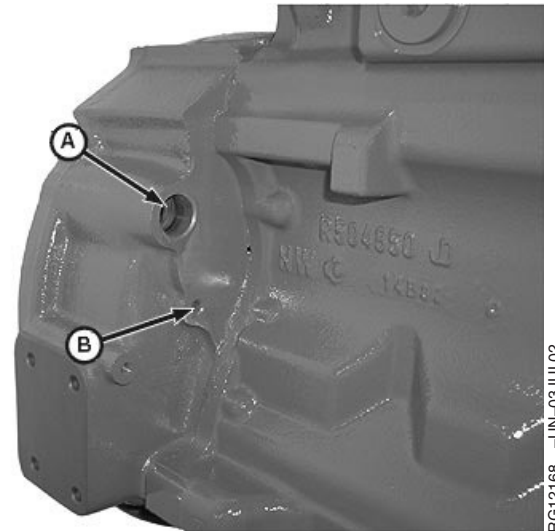
Flywheel Housing Timing Holes
