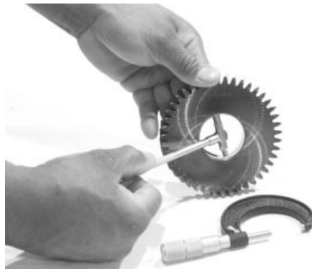
Measuring Idler Gear Bushing ID
