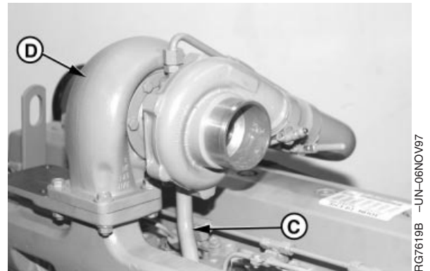
Connect Turbocharger Lines
