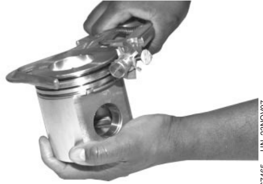
Cleaning Piston Ring Grooves
