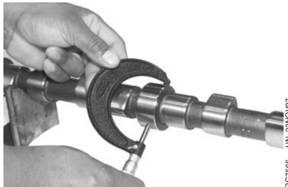
Measuring Camshaft Journal OD
