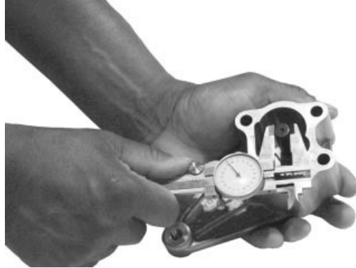
Measure Idler Shaft OD for Wear
