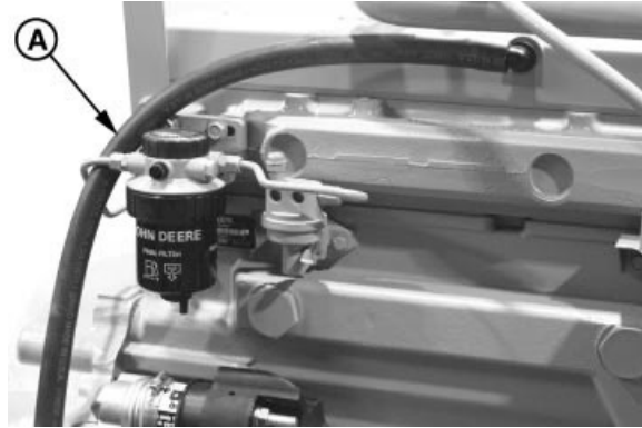
Ventilator Outlet Hose Inspection
