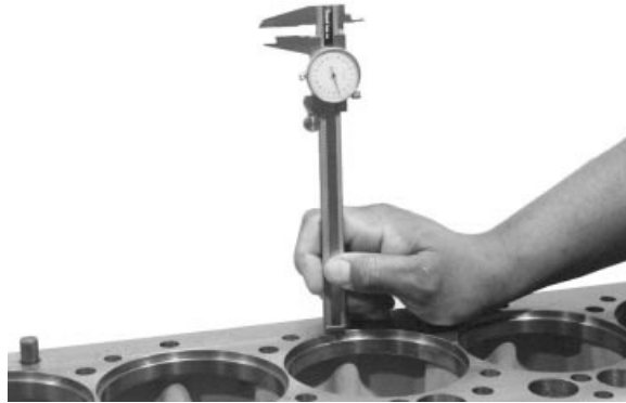
Measure Liner Flange Counterbore Depth
