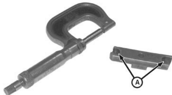
Inspect and Measure Bridges
