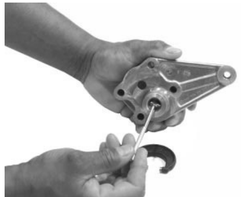
Measuring Bushing ID in Housing for Wear
