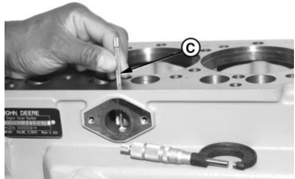
Push Rod Bore in Block Wear
