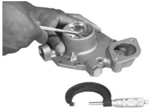
Coolant Pump Housing Weep Hole
