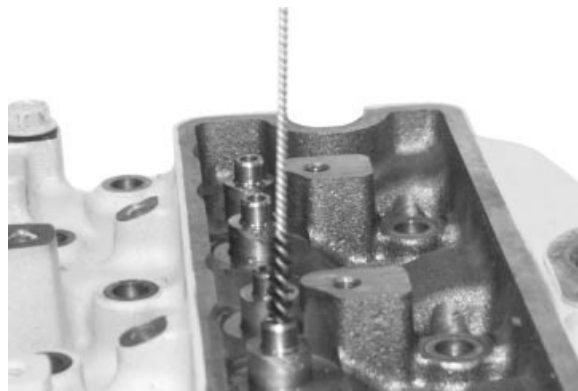
Valve Guide Cleaning
