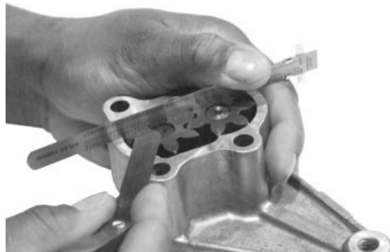
Checking Gear-to-Pump Cover Axial Clearance
