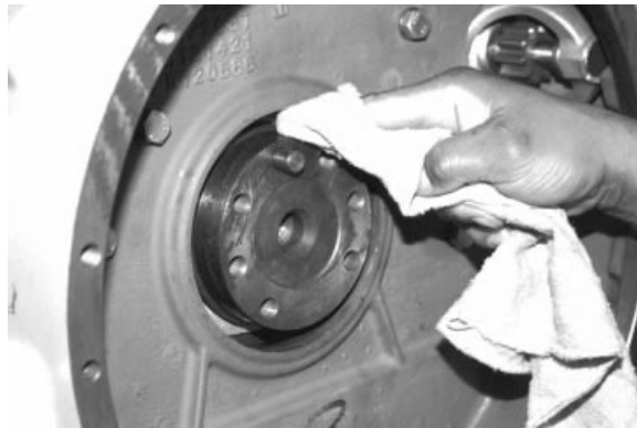
Clean Crankshaft Flange
