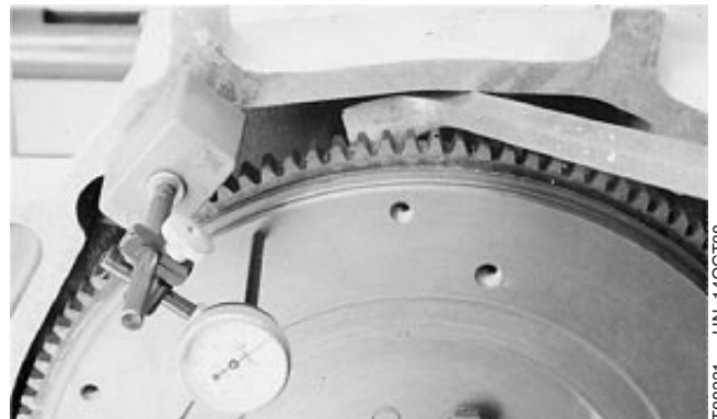
Check Crankshaft End Play w/Dial Indicator
