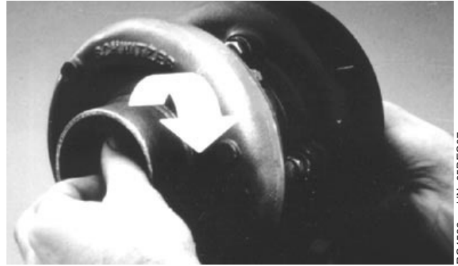
Checking Shaft Rotation and Clearance
