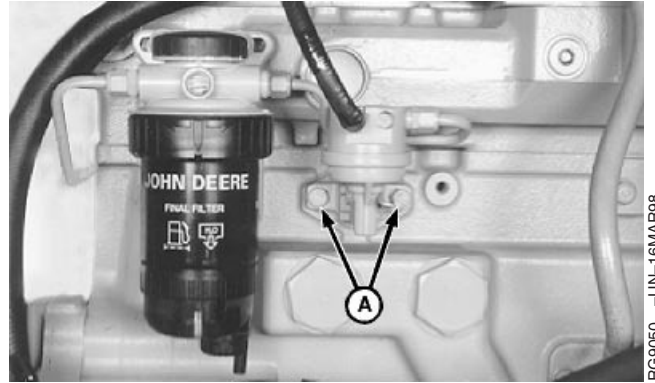
Fuel Supply Pump
