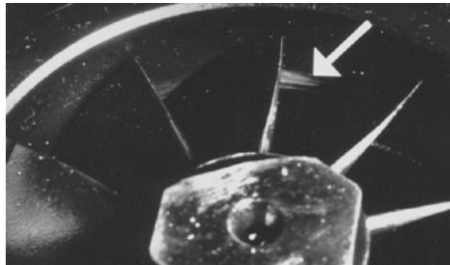
Checking Turbine Wheel Blades
