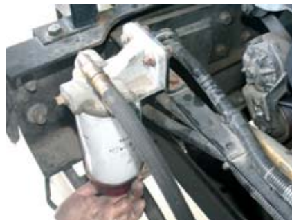
This water separator can be drained from the bottom; note the hand underneath.
