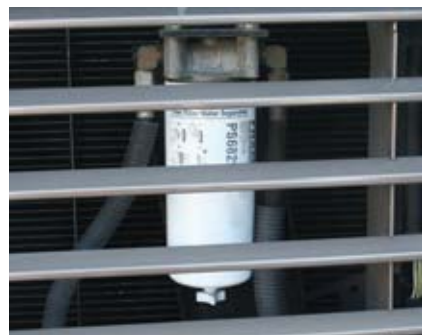
Note the drain valve knob on the bottom of this filter. Place a catch pan underneath before opening.
