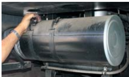
Note the drain valve knob on the bottom of this filter. Place a catch pan underneath before opening.
