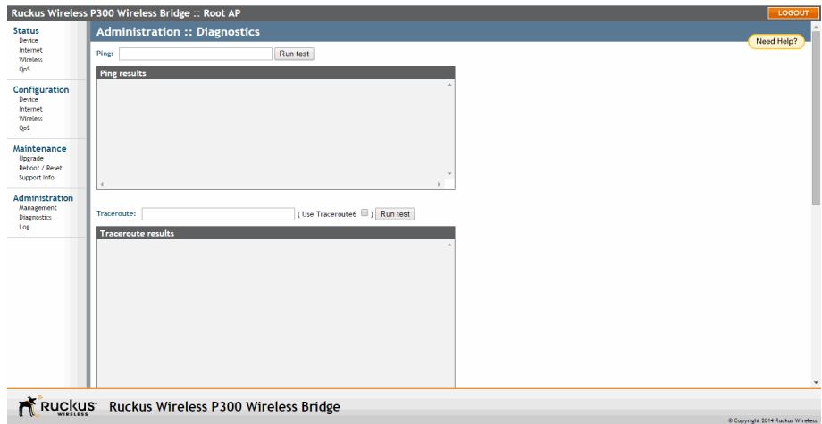
Figure 36. Using ping or traceroute
