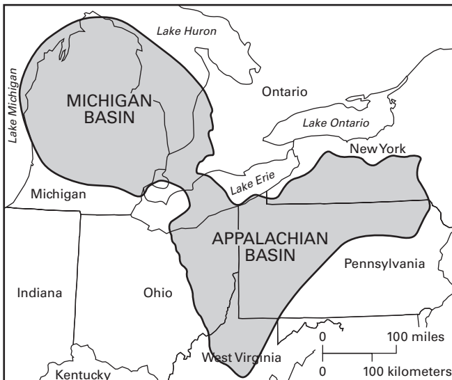
Extent of the salt-bearing Salina Group in the Appalachian and Michigan Basins (from Hansen, 1983).
