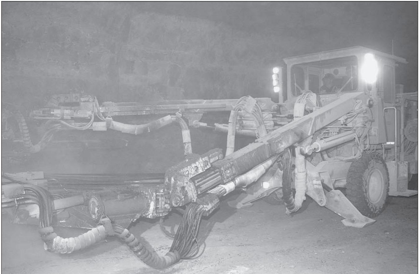
A Cannon twin-boom jumbo drill is operated by John Bergles at the East Fairfield Coal Co. underground limestone mine in Mahoning County. The drill is capable of drilling 56 holes, 16 feet deep, in 1 hour and 10 minutes. Horizontal and vertical angles of the drill holes can be varied to facilitate blasting. Water from an attached tank is used to remove the drill cuttings and to control dust.
