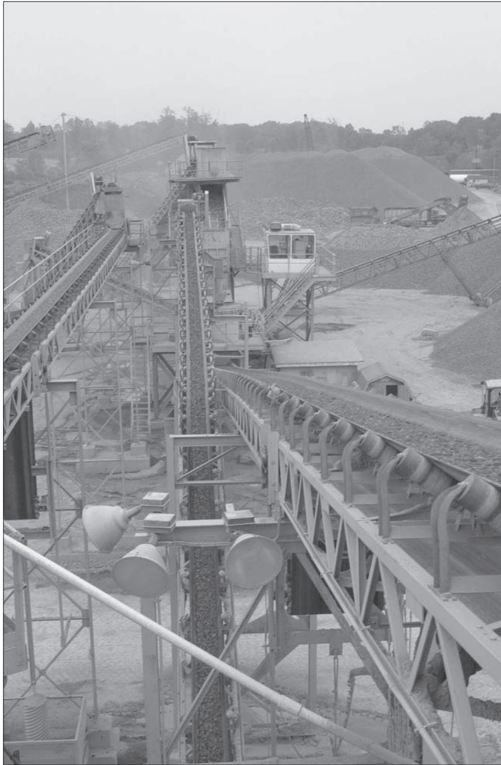
The aggregate processing plant at the East Fairfield Coal Co. limestone mine in Mahoning County. The beltlines carry product from the primary crusher to the wet screen and the oversize ( >2\frac{1}{2} inches) is carried back for recrushing.
