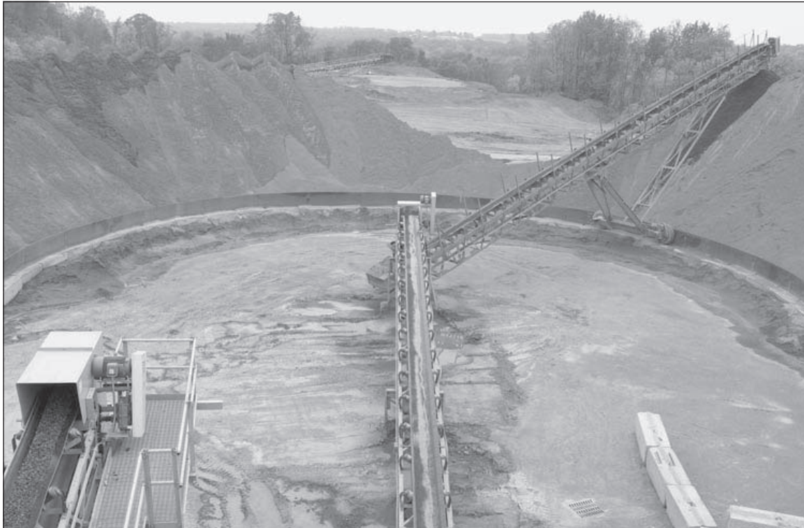
Manufactured sand used in asphalt, concrete block, and pipe fill is being conveyed to storage at the processing facilities of the East Fairfield Coal Co. limestone mine in Mahoning County.
