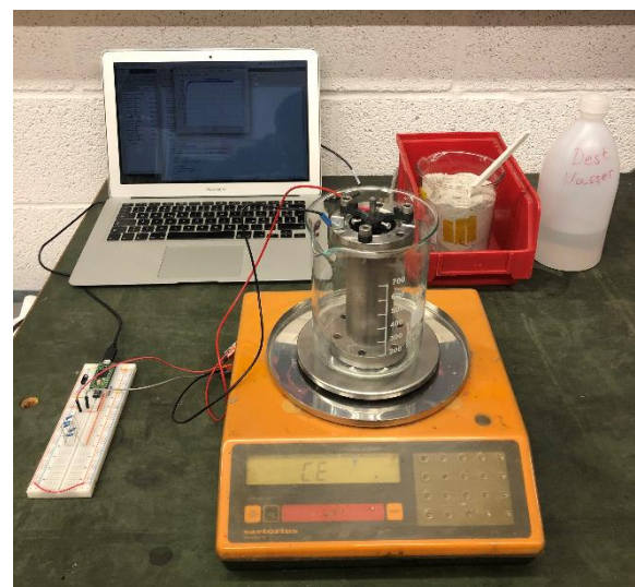
Figure 2: Experimental Setup: LVS system connected to read-out electronics and on precision scale. Quartz sand and distilled water in the background.
