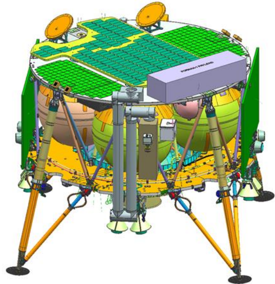
Fig. 1: Configuration of LSAS lander with payload of first mission accommodated
