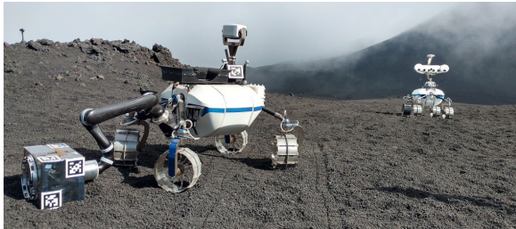
Figure 1: Team of our Lightweight Rover Units (LRUs) [4] at a Moon-analogue site on Mt. Etna
