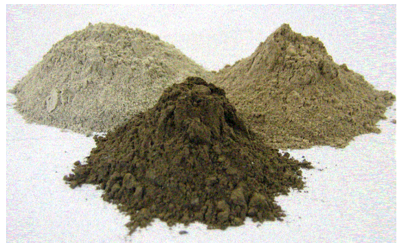
Fig. 2: Components of the modular regolith simulant system for the processing of the required simulants
