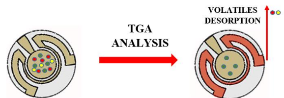
Figure 1: Volatiles desorption from PCM by using the built-in RTD.
