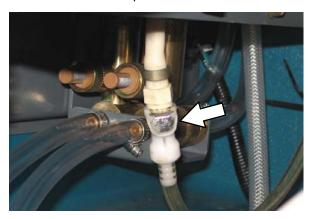
4. Remove the perforated knock outs from the new FaST-PAK carton. Do Not remove the bag from the carton. Pull out the hose connector located on the bottom of the bag and remove the hose cap from the connector.
