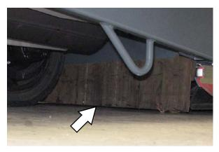
The skirts should be between 0 to 6 mm (0 to 0.25 in) from the floor when the scrub head is down.
