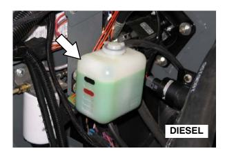
Flush the radiator and the cooling system after every 800 hours of operation.
