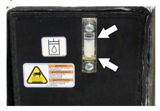
ATTENTION! Do not overfill the hydraulic fluid reservoir or operate the machine with a low level of hydraulic fluid in the reservoir. Damage to the machine hydraulic system may result.
