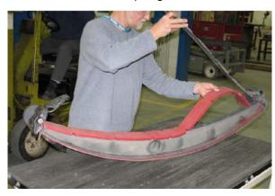
13. Install the new front squeegee blade or rotate the existing blade to the new edge. Be sure the holes in the squeegee blade are hooked onto the tabs.
