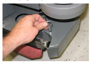
3. Remove the clevis pin and squeegee retainer.
