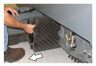
6. Install the new or rotated brushes by pushing down on the ends while sliding them onto the drive motor hubs.
