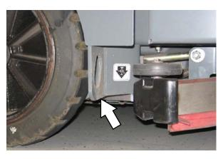
Front jacking locations are located on the frame directly in front of the front tire.
