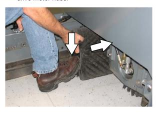
7. If rotating the existing brushes, only rotate front to rear. Do NOT rotate end-for-end.
