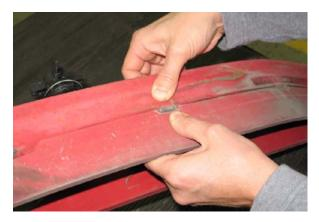
9. Reinstall the rear retaining band aligning the tabs with the holes.
