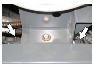
On the other side of the machine the torque tube grease fittings are located beneath the propel pump.
