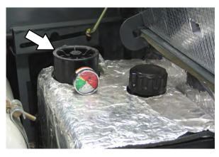
Replace the hydraulic strainer outlet after every 2400 hours of operation.
