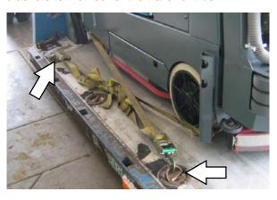
10. If the loading surface is not horizontal or is higher than 380 mm (15 in) from the ground, use a winch to unload machine.
