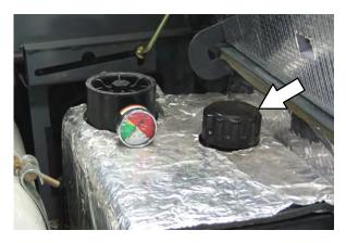
Replace the hydraulic fluid filter after every 1200 hours of operation or if the hydraulic reservoir gauge is in the yellow/red zone when the reservoir hydraulic fluid is approximately 32° C (90° F).
