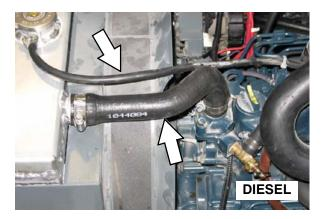
Check the radiator core exterior and hydraulic cooler fins for debris after every 100 hours of operation. Blow or rinse all dust through the grille and radiator fins, in the opposite direction of normal air flow. Be careful to not bend the cooling fins when cleaning. Clean thoroughly to prevent the fins from becoming encrusted with dust. To avoid cracking the radiator, allow the radiator and cooler fins to cool before cleaning.
