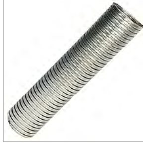
01338128 PIPE,EXHAUST,FLEX,3.00 ID,14 IN LG TCFE
