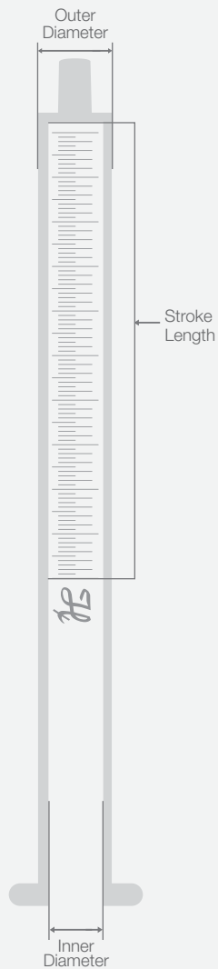
Syringes Figure 7. Syringe dimensions
