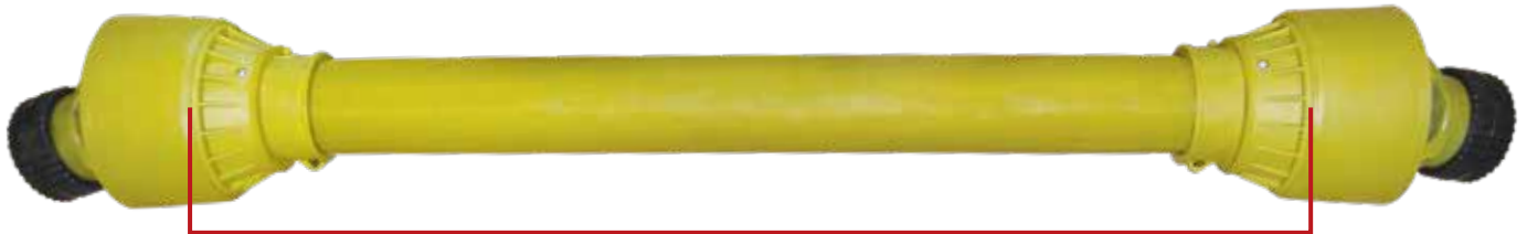
L (COLLAPSED LENGTH)
