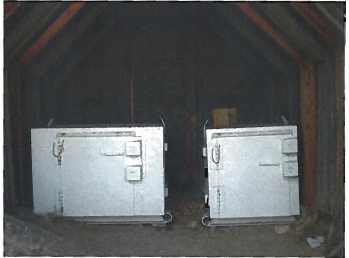
Magazines for Primers (replaced storage sheds)
