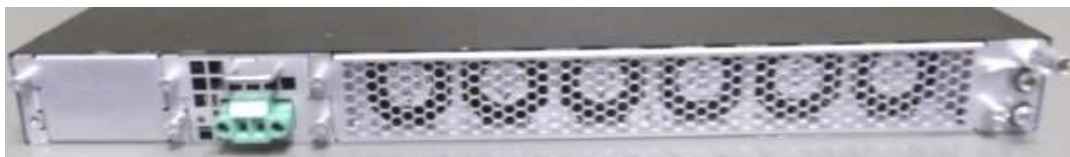
Figure 40 NI-CER-2024F-ADVPREM-DC backside with Interface module: NI-CER-2024-2X10G with Power supply: RPS9DC (DC Power Supply)
