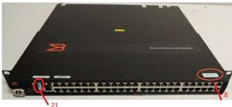
Figure 89 Front, top view of a Brocade NetIron CER 2048 device with security seals
