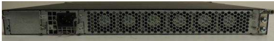
Figure 38 NI-CER-2024F-ADVPREM-AC backside with Interface module: NI-CER-2024-2X10G with Power supply: RPS9 (AC Power Supply)
