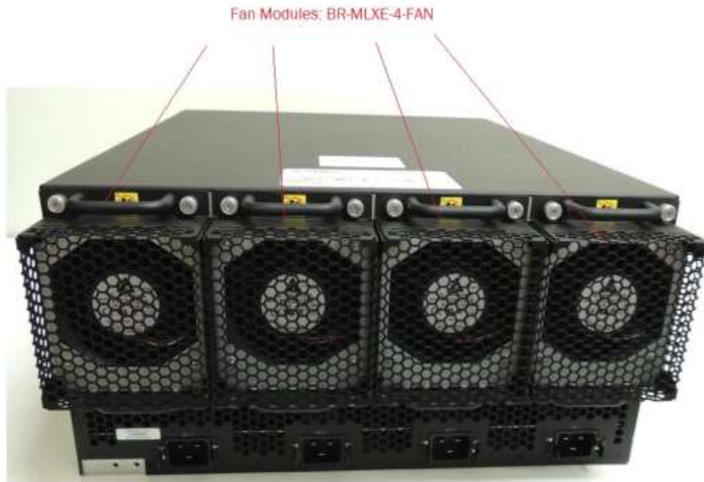
Figure 4 MLXe-4 Cryptographic Module with Chassis: BR-MLXE-4-MR-M-DC backside
