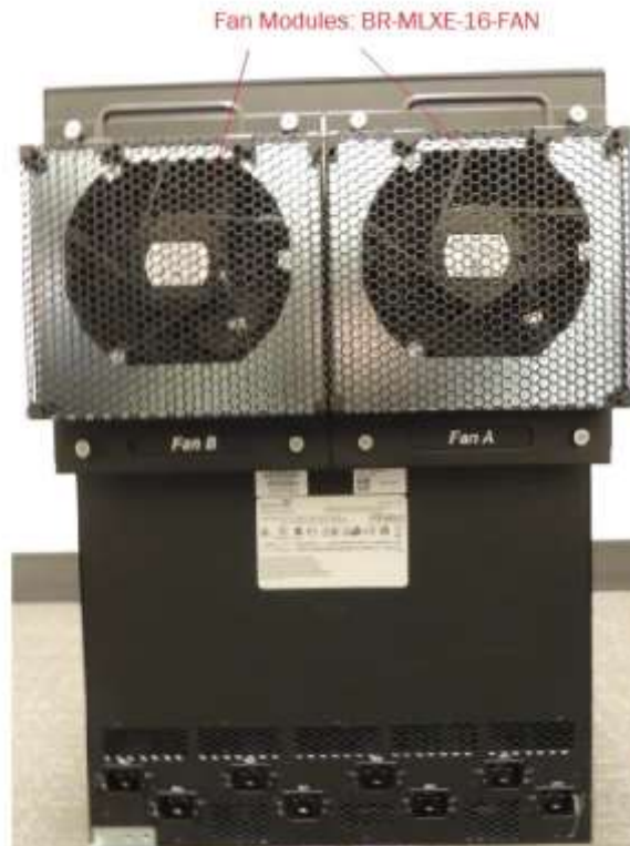
Figure 22 MLXe-16 Cryptographic Module with Chassis: BR-MLXE-16-MR2-M-AC backside
