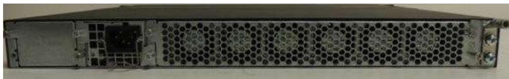
Figure 26 NI-CER-2048F-ADVPREM-AC backside with Power supply: RPS9 (AC Power supply)
