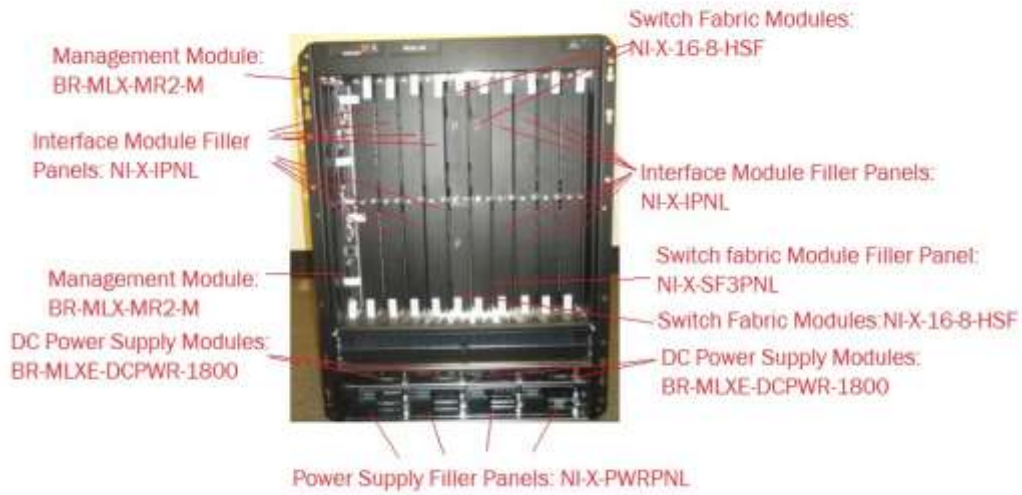
Figure 23 MLXe-16 Cryptographic Module with Chassis: BR-MLXE-16-MR2-M-DC (DC Power Supply)
