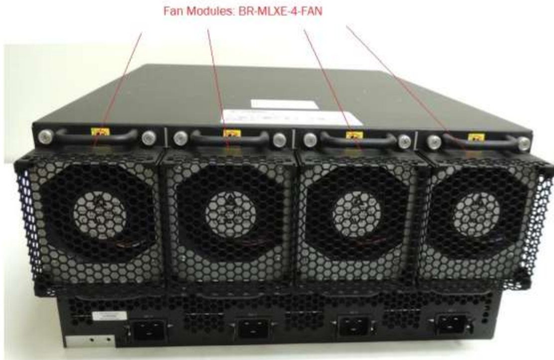
Figure 8 MLXe-4 Cryptographic Module with Chassis: BR-MLXE-4-MR2-M-DC backside
