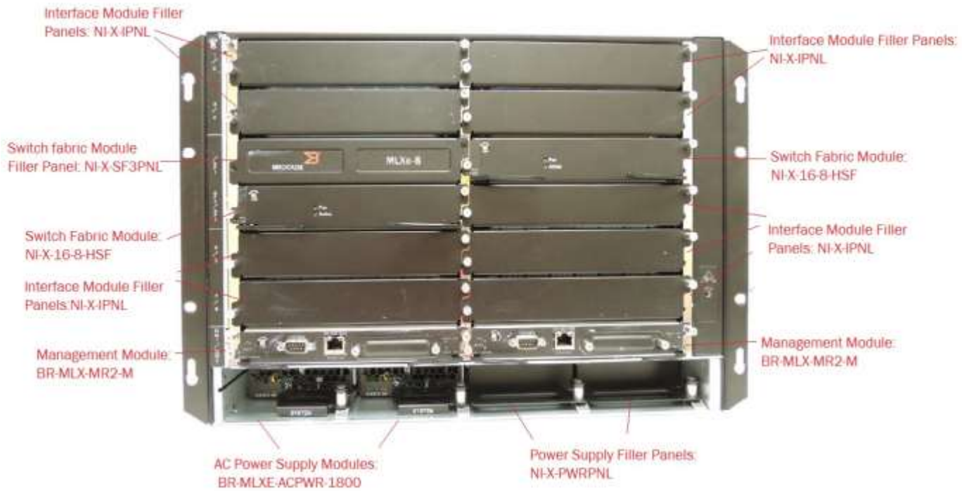
Figure 13 MLXe-8 Cryptographic Module with Chassis: BR-MLXE-8-MR2-M-AC (AC Power Supply)
