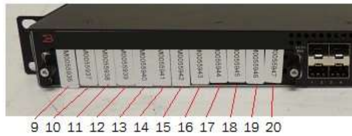
Figure 86 Rear, top and left side view of a Brocade NetIron CER 2024F device with security seals
