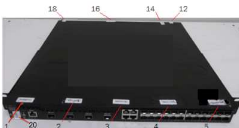
Figure 102 Top front view of a Brocade CES 2024C-4X device with security seals
