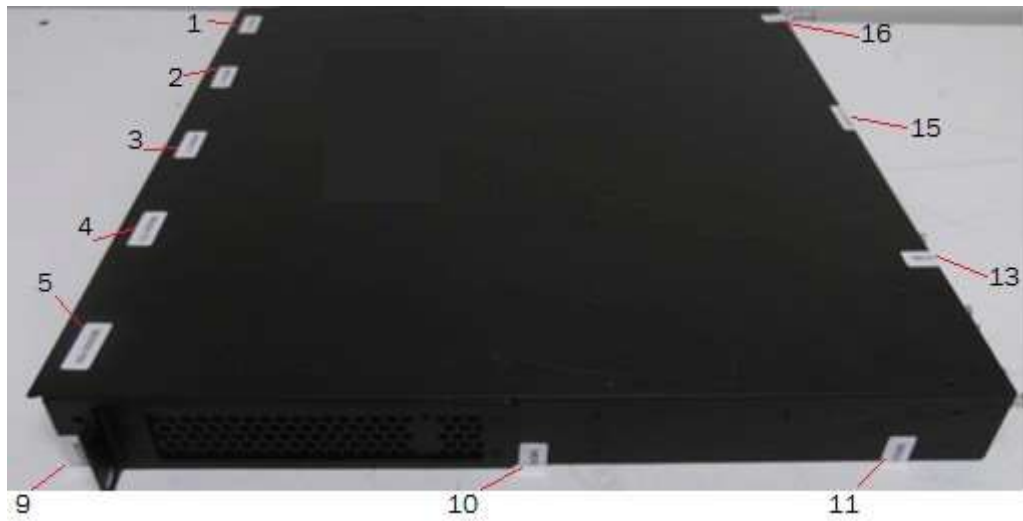
Figure 94 Left side view of a Brocade CER 2024C-4X-RT device with security seals
