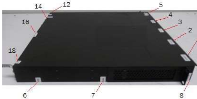
Figure 109 Left side view of a Brocade CES 2024F-4X device with security seals
