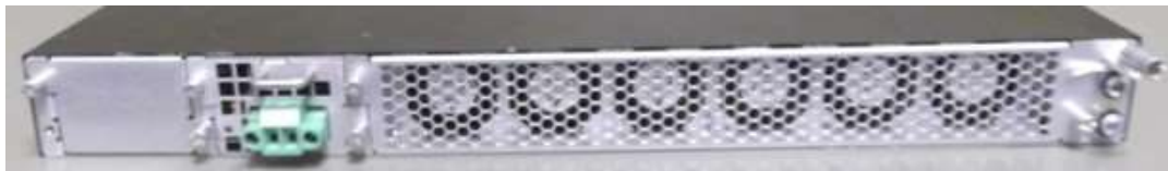
Figure 68 BR-CES-2024C-4X-DC backside with Power supply: RPS9DC (DC Power supply)
