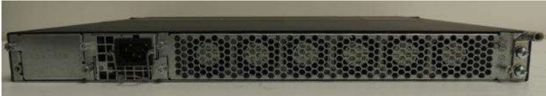
Figure 42 NI-CER-2024C-ADVPREM-AC backside with Power supply: RPS9 (AC Power supply)
