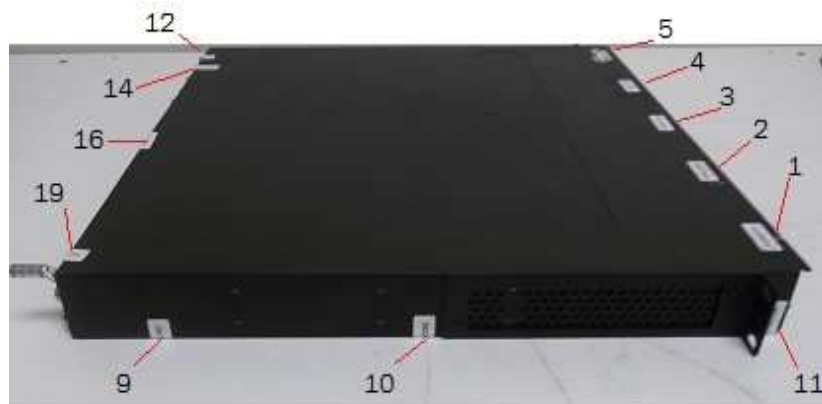
Figure 100 Rear view of a Brocade CER 2024F-4X-RT device with security seals
