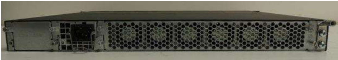
Figure 47 NI-CER-2024C-ADVPREM-DC with Base: NI-CER-2024C-DC, Interface module: NI-CER-2024-2X10G and License: SW-CER-2024-ADVU
