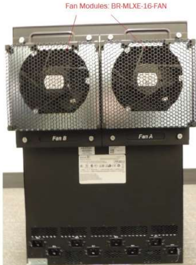
Figure 20 MLXe-16 Cryptographic Module with Chassis: BR-MLXE-16-MR-M-DC backside
