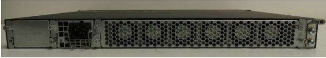
Figure 70 BR-CES-2024F-4X-AC backside with Power supply: RPS9 (AC Power supply)
