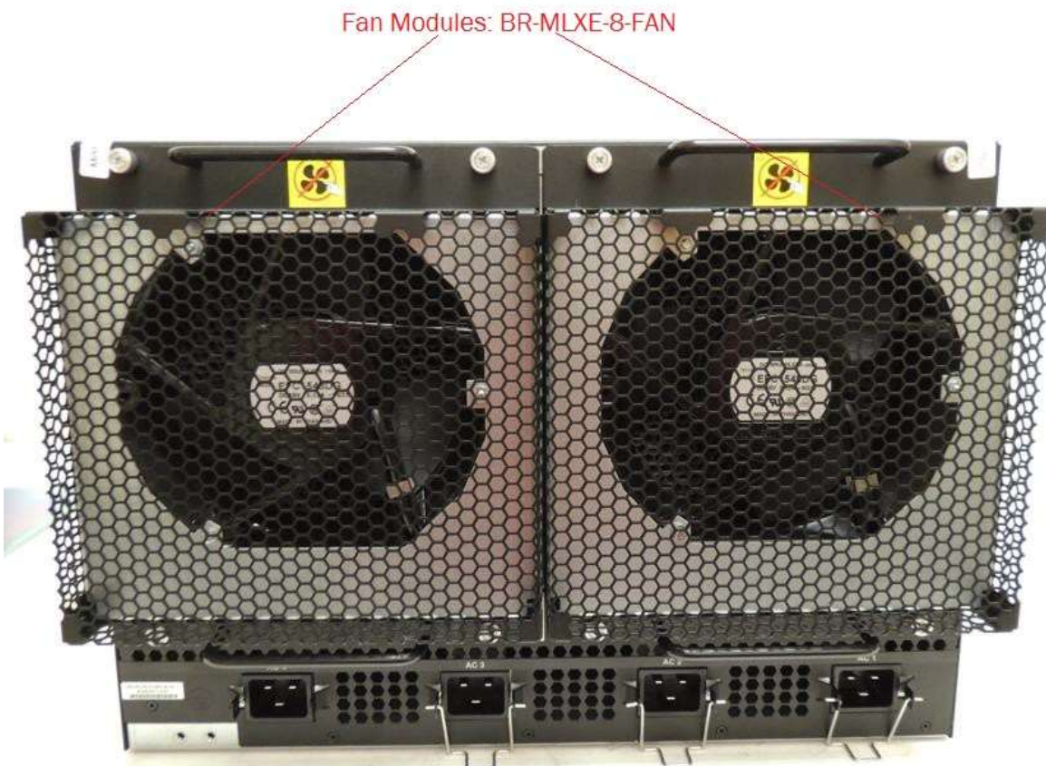
Figure 12 MLXe-8 Cryptographic Module with Chassis: BR-MLXE-8-MR-M-DC backside
