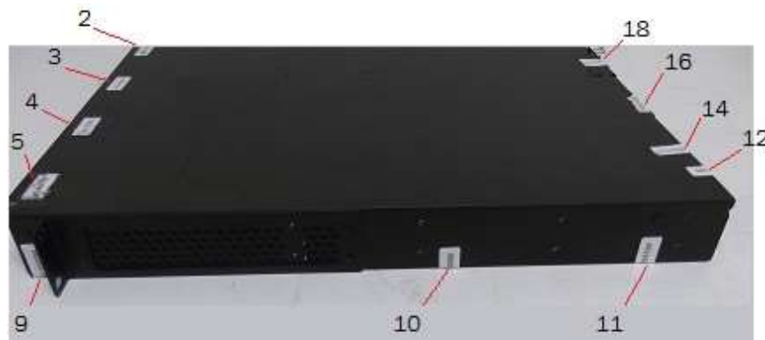
Figure 103 Right side view of a Brocade CES 2024C-4X device with security seals
