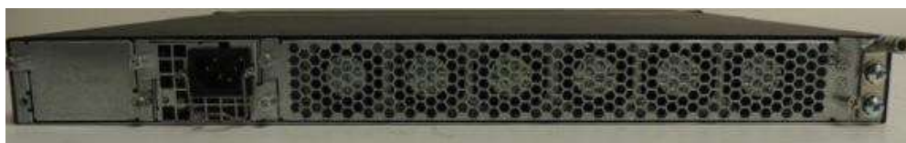
Figure 30 NI-CER-2048FX-ADVPREM-AC backside with Power supply: RPS9 (AC Power Supply)
