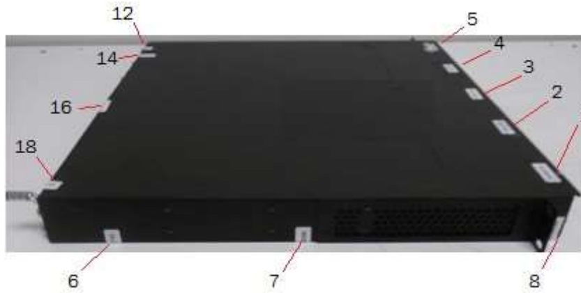
Figure 104 Left side view of a Brocade CES 2024C-4X device with security seals
