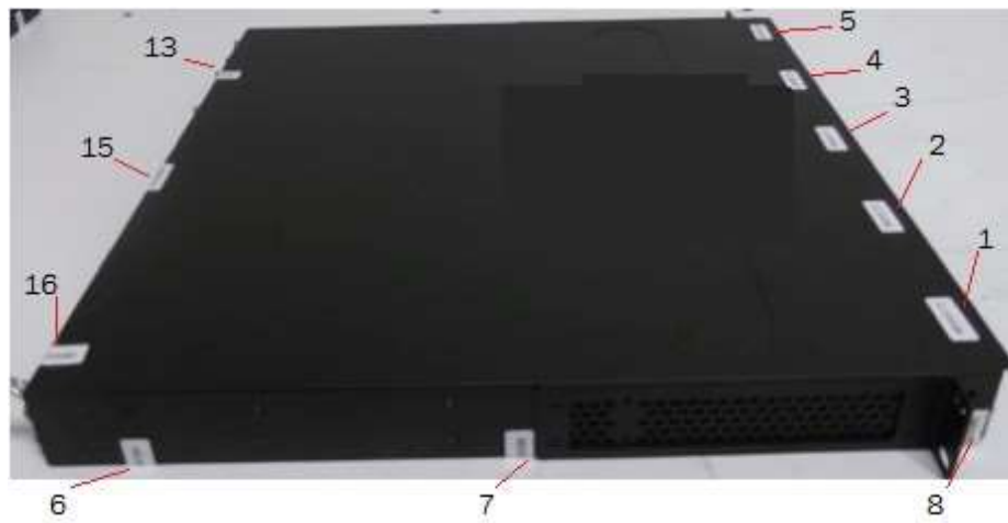
Figure 94 Left side view of a Brocade CER 2024C-4X-RT device with security seals
