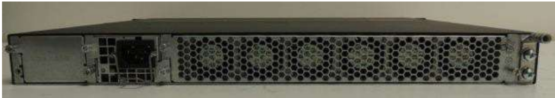
Figure 66 BR-CES-2024C-4X-AC backside with Power supply: RPS9 (AC Power supply)
