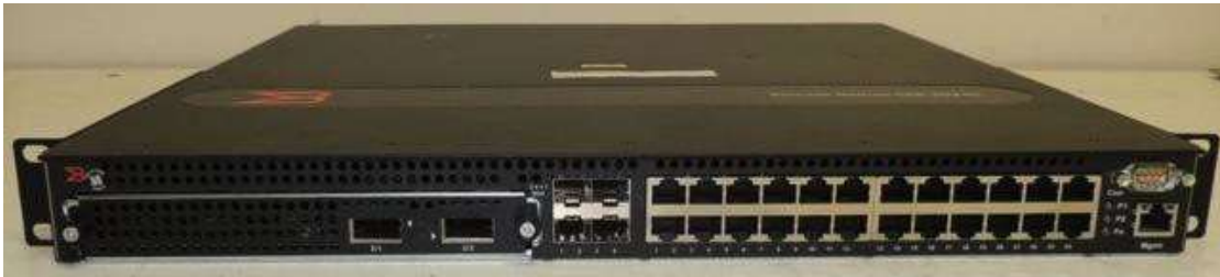
Figure 48 NI-CER-2024C-ADVPREM-DC backside with Interface module: NI-CER-2024-2X10G with Power supply RPS9DC (DC Power Supply)
