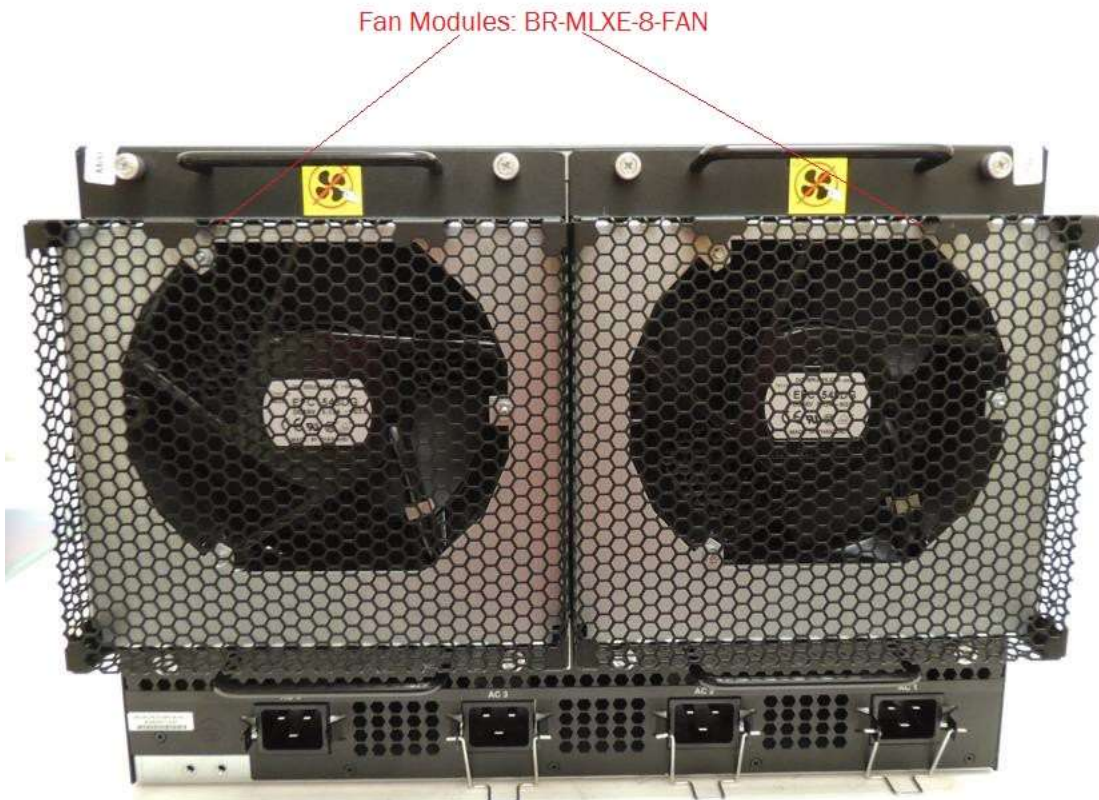
Figure 14 MLXe-8 Cryptographic Module with Chassis: BR-MLXE-8-MR2-M-AC backside
