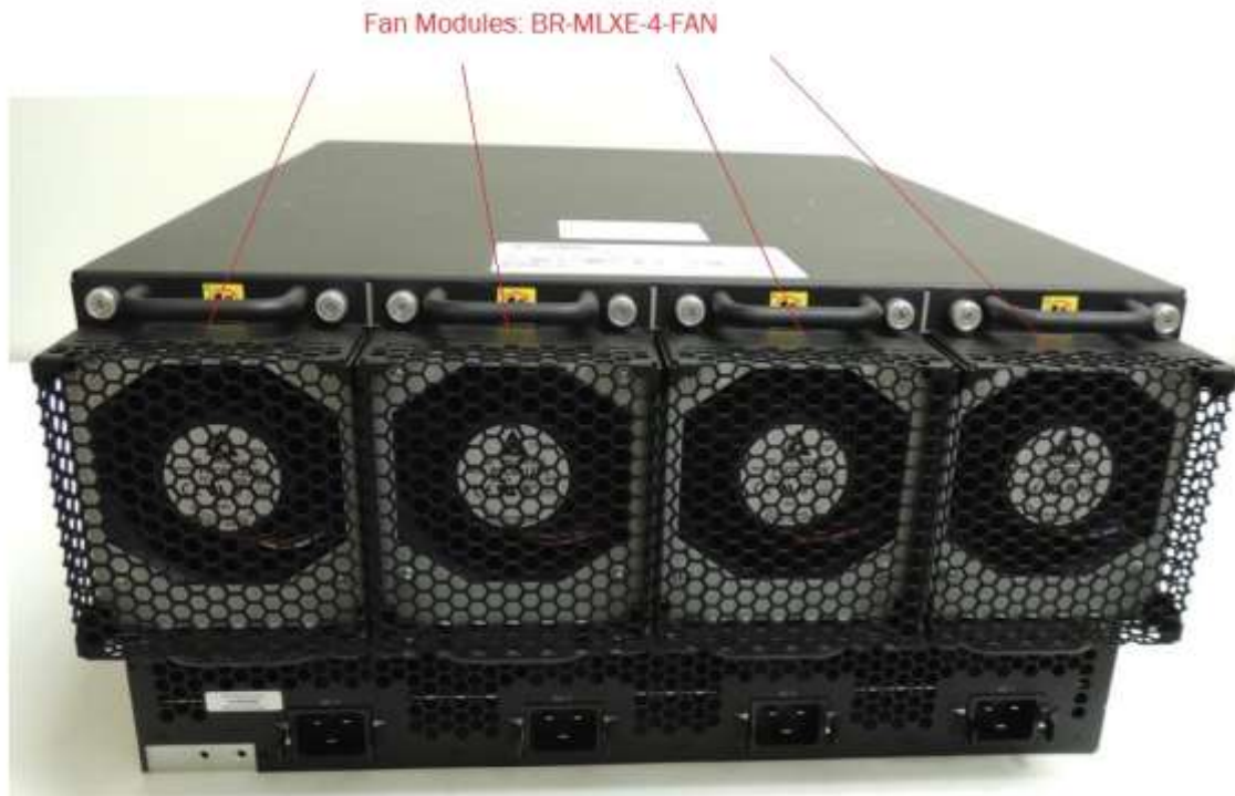
Figure 6 MLXe-4 Cryptographic Module with Chassis: BR-MLXE-4-MR2-M-AC backside
