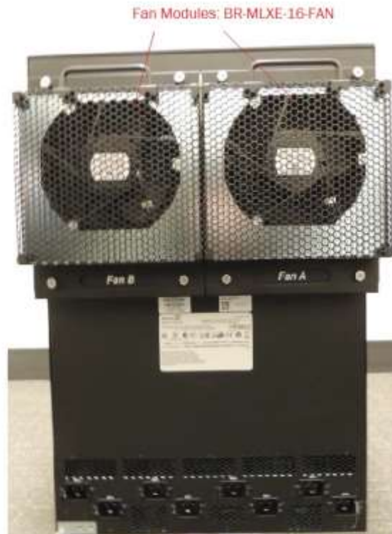
Figure 18 MLXe-16 Cryptographic Module with Chassis: BR-MLXE-16-MR-M-AC backside
