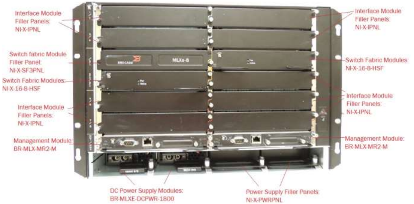
Figure 16 MLXe-8 Cryptographic Module with Chassis: BR-MLXE-8-MR2-M-DC backside
