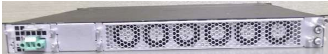
Figure 60 BR-CER-2024C-4X-RT-DC backside with Power supply RPS9DC (DC Power Supply)
