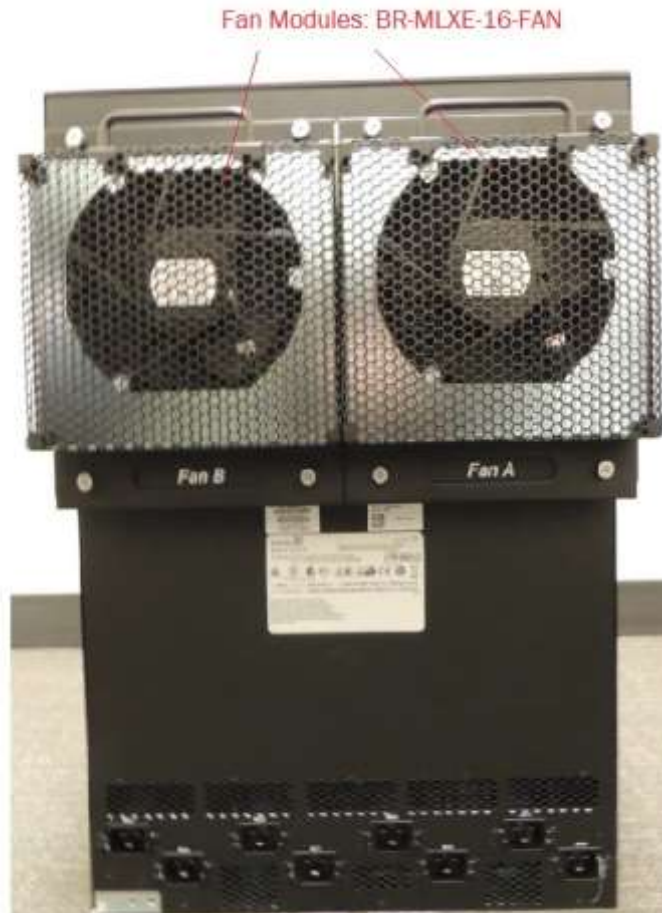
Figure 24 MLXe-16 Cryptographic Module with Chassis: BR-MLXE-16-MR2-M-DC backside
