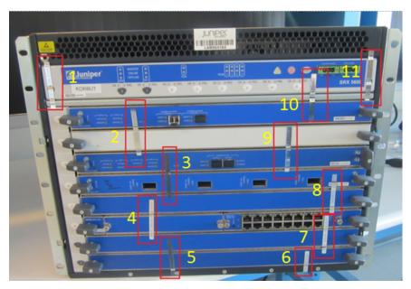
Figure 11 - SRX5600- Tamper-Evident Seal Locations on Front- 11 Seals
