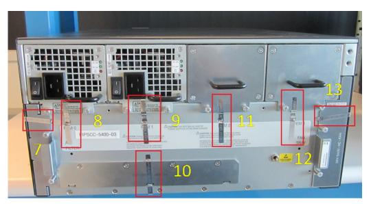
Figure 10 - SRX5400- Tamper-Evident Seal Locations on Rear- Seven Seals
