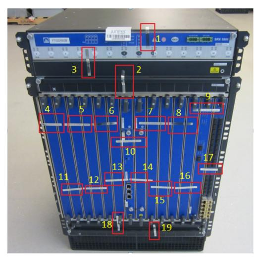
Figure 13 - SRX5800- Tamper-Evident Seal Locations on Front- 19 Seals
