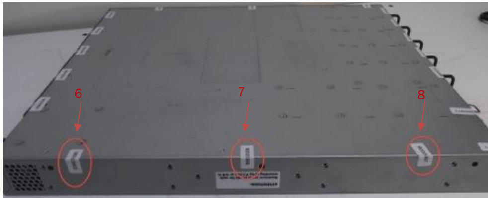
Figure 14 - VDX 6740T-24, VDX 6740T-48, VDX 6740T-64 and VDX 6740T-56-1G bottom left side seal locations
