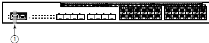
Figure 52 - ICX6610-24F - Front view with tamper evident label security seals
