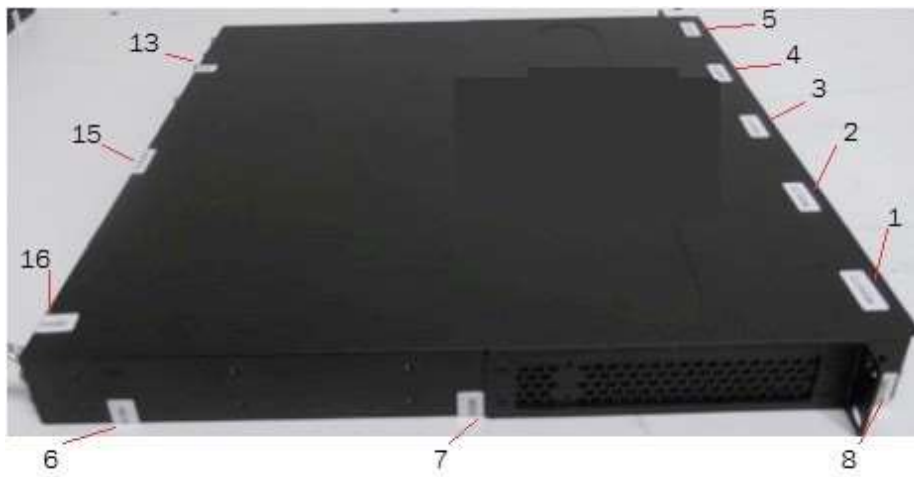
Figure 94 Left side view of a Brocade CER 2024C-4X-RT device with security seals
