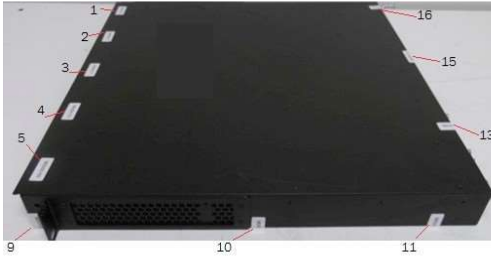
Figure 93 Right view of a Brocade CER 2024C-4X-RT device with security seals
