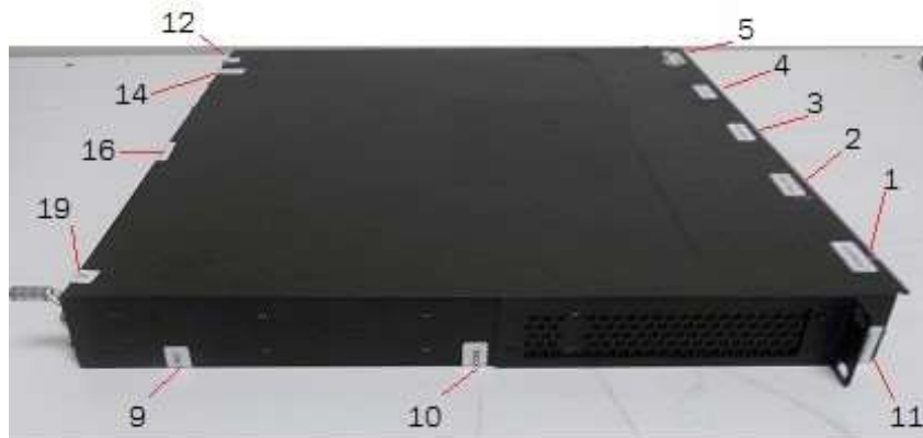
Figure 99 Left view of a Brocade CER 2024F-4X-RT device with security seals
