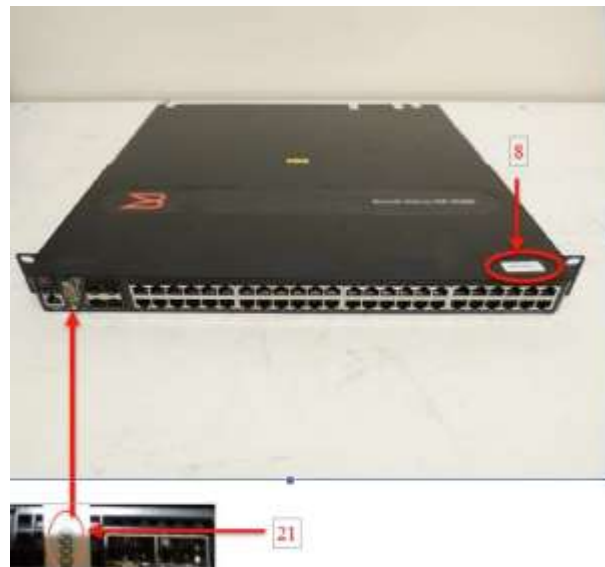
Figure 89 Front, top view of a Brocade NetIron CER 2048 device with security seals
