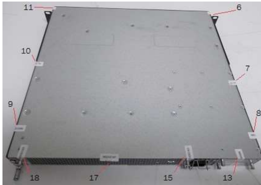
Figure 101 Bottom view of a Brocade CER 2024F-4X-RT device with security seals
