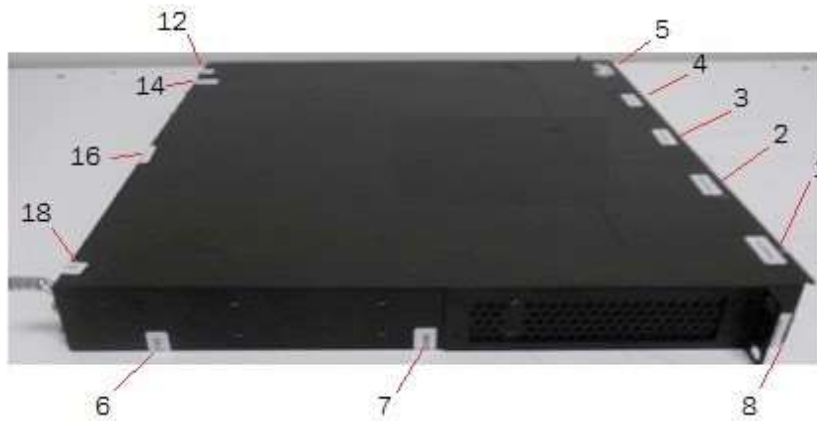
Figure 104 Left side view of a Brocade CES 2024C-4X device with security seals
