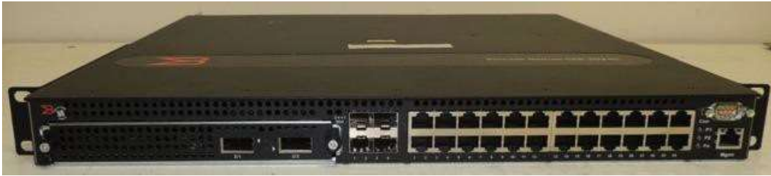
Figure 46 NI-CER-2024C-ADVPREM-AC backside with Interface module: NI-CER-2024-2X10G with Power supply RPS9 (AC Power Supply)
