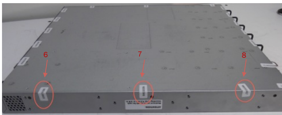
Figure 25 VDX 6740T-24, VDX 6740T-48, VDX 6740T-64 and VDX 6740T-56-1G bottom left side seal locations
