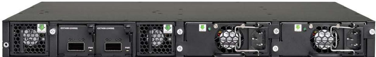
Figure 3 - Back side of ICX7450-48P with IPsec module inserted
