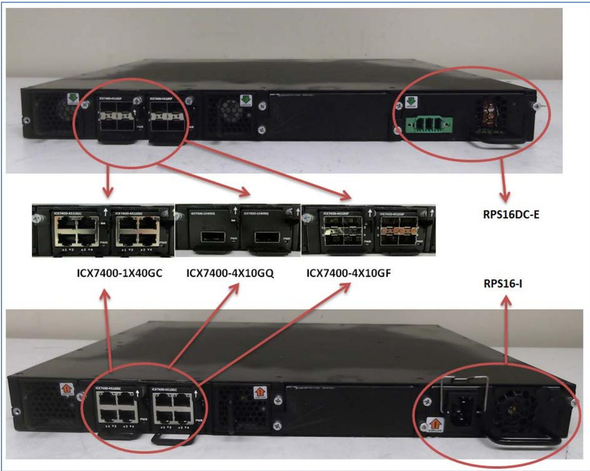
Figure 7 - Back side of the module ICX7450-48P with ICX7400-1X40GC, ICX7400-4X10GQ and ICX7400-4X10GF
