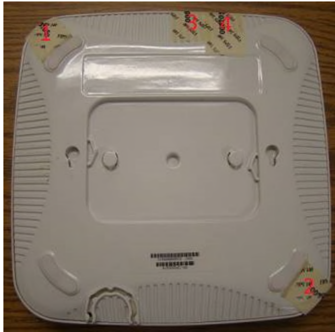
Figure 10 - Required TELs for the Aruba 7005 Mobility Controller – Bottom
