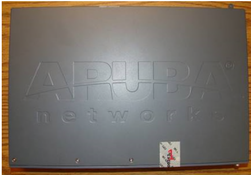
Figure 24 - Required TELs for the Aruba 7205 Mobility Controller – Top
