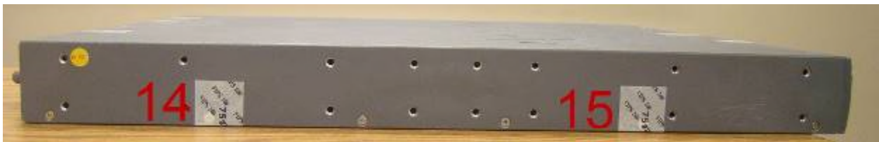
Figure 31 - Required TELs for the Aruba 7200 Mobility Controller – Left Side
