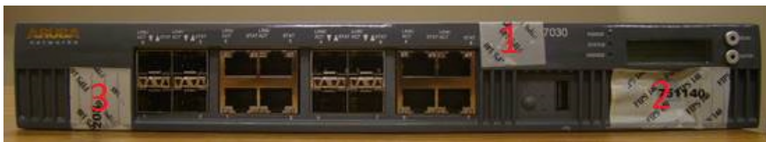
Figure 22 - Required TELs for the Aruba 7030 Mobility Controller – Front
