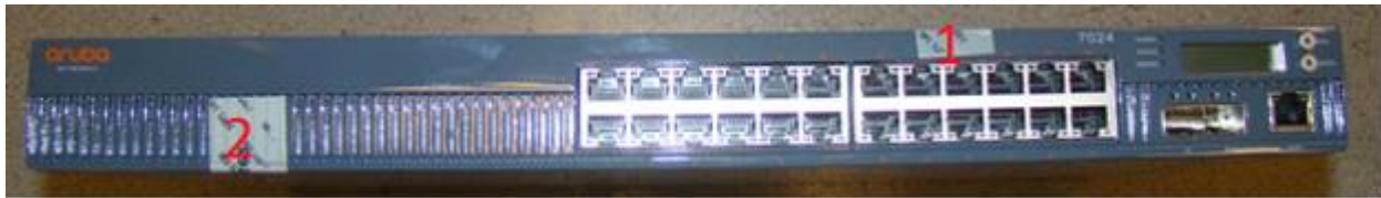
Figure 17 - Required TELs for the Aruba 7024 Mobility Controller – Front
