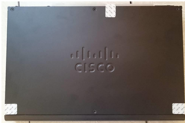
Figure 35 ASA 5508-X Top TEL Placement
