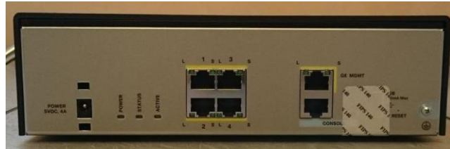
Figure 28 ASA 5506H-X Rear TEL Placement
