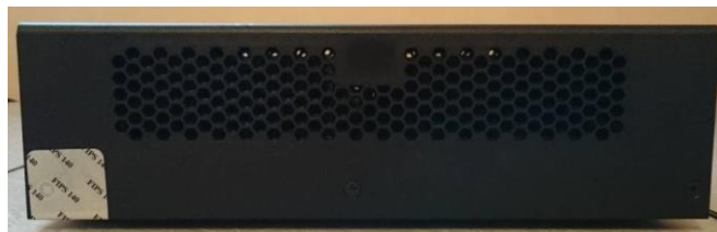
Figure 26 ASA 5506H-X Right Side TEL Placement
