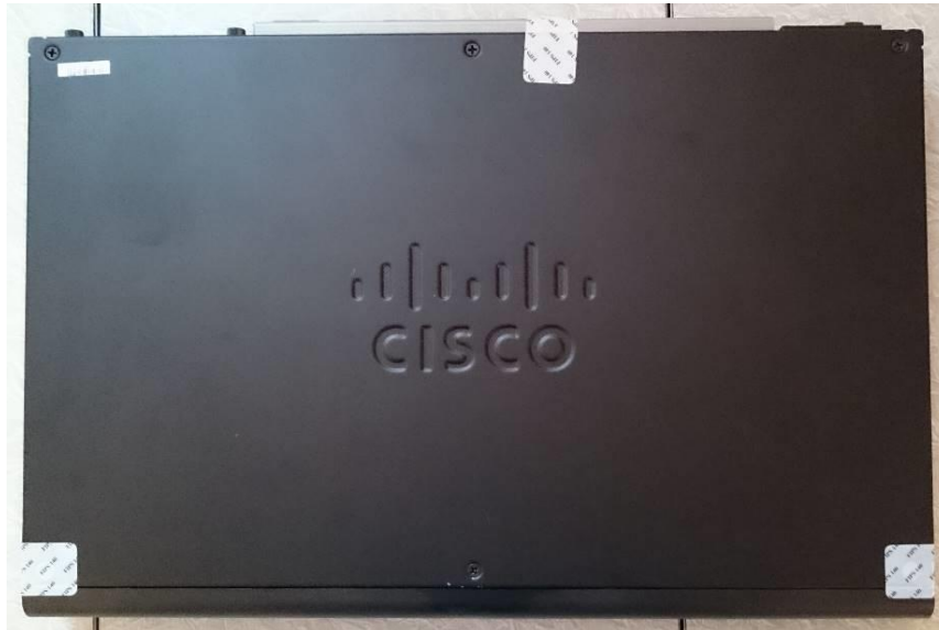
Figure 41 ASA 5516-X Top TEL Placement
