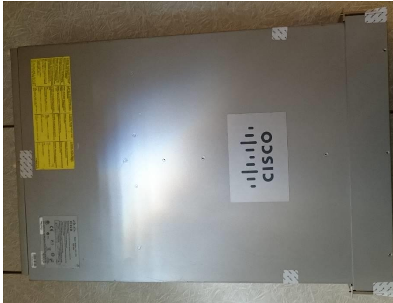
Figure 65 ASA 5585-X Top TEL Placement
