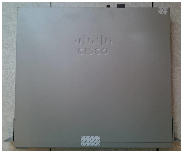
Figure 47 ASA 5525-X Top TEL Placement
