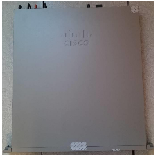
Figure 59 ASA 5555-X Top TEL Placement
