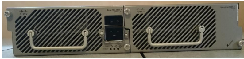
Figure 64 ASA 5585-X Rear View
