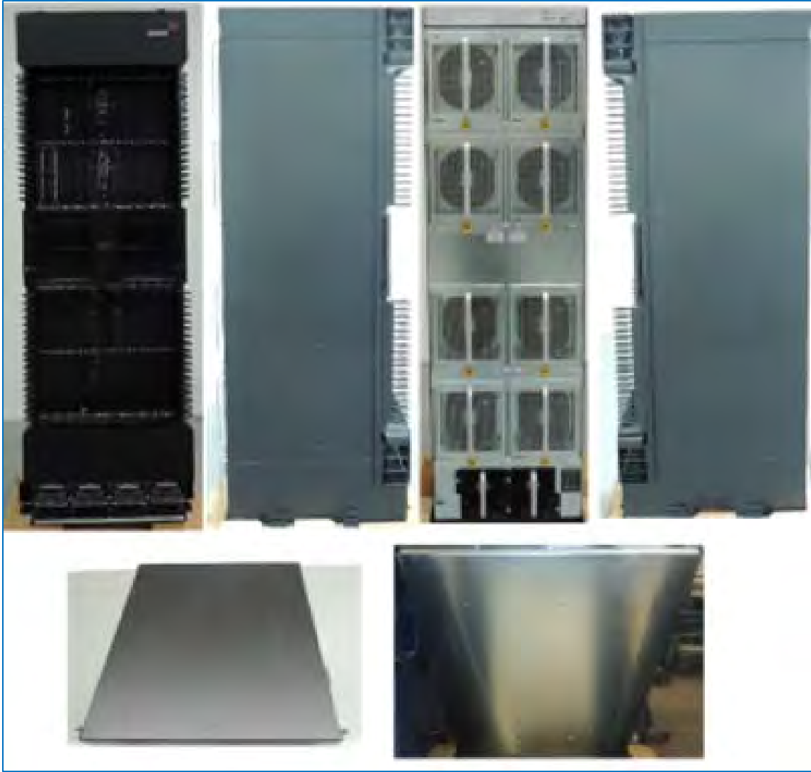
Figure 9 – Brocade MLXe-32: Starting from left to right clockwise: Front side, Left side, Rear side, Right side, Bottom side, and Top side
