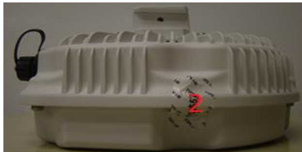
Figure 19 – Right Side View of AP-277 with TELs
