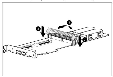
Reinstall the controller in the server.
