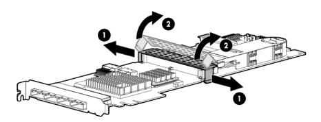
Δ **CAUTION:** When connecting or disconnecting the capacitor pack cable, the connectors on the cache module and cable are susceptible to damage. Avoid excessive force and use caution to avoid damage to these connectors.
