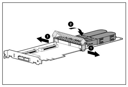
Swivel the latches on the DIMM connector outward (1).
