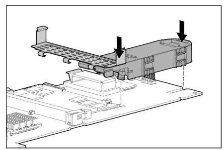
Δ **CAUTION:** When connecting or disconnecting the capacitor pack cable, the connectors on the cache module and cable are susceptible to damage. Avoid excessive force and use caution to avoid damage to these connectors.
