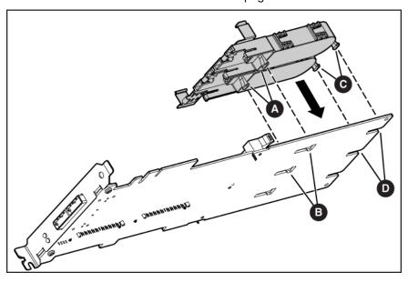
Slide the batteries toward the board bracket until they are firmly seated against the connectors on the cache module.
