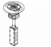
The Poke Thru Series by Legrand/Wiremold is used to bring power and communications services to the open-space areas of your work environment.
