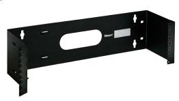
Mounts to wall or standard EIA 19 in. rack. Includes cable tie slots. Has standard 19 in. EIA hole spacing. Panel rotates from one side for easy access to cabling. Includes write-on labeling area and accepts 19 in. patch panels, horizontal cable managers and equipment.
