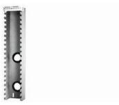
The Type 85 Mounting Bracket accepts 8-pair Series 2 blocks. The stainless steel bracket comes with cable entry holes on the back and protective rubber grommets. All holes are 1.375 in. (35 mm) in diameter. (NOTE: When mounting directly to a wall, do not install rubber grommets.)
