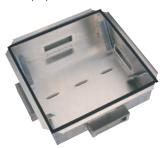
This raised floor enclosure provides easy access to a rack-mount fiber enclosure when it is located under a raised floor. Placing connections under the raised floor saves valuable rack-mount space within equipment cabinets and allows the data center to be easily reconfigured - just unplug the patch cords and move the cabinet. The fiber enclosure is placed under a 2 ft. x 2 ft. raised floor tile. The enclosure is 8 in. high and can be installed in raised floors that are at least 9 in. high.
