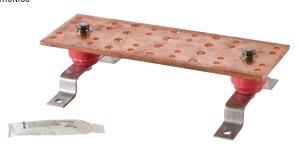
Manufactured of 1/4 in. thick electrolytic tough pitch 110 alloy copper bar. Includes  $1\,1/2$  in. insulators and 1 in. off-set stainless steel mounting brackets. Includes one 1/2 oz. tube of antioxidant joint compound. Meets BICSI and EIA/TIA 607 standards.
