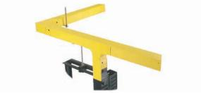
The FIBER-DUCT Routing System is a complete fiber optic cable routing system that can be used for all fiber optic cabling installations. Used in telecommunications closets, equipment rooms or in approved underfloor applications. The channel comes with standard mounting holes. The specially designed fittings feature a minimum 2 in. bend radius to protect fiber optic cables. The channel and fittings are made from V-O flame class-rated materials.
