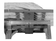
Secures cable runway to the top of Standard and Universal equipment racks. J-bolts hook under the mounting plate to secure the plate to the rack's top angles. Mounts either parallel or perpendicular.
