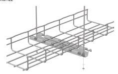
For trapeze-hung installations or use on walls, floors and cabinets. Patented FAS-style attachments holds cable tray secure without nuts and bolts. For trapeze-hung installations, use 4 in. longer profile than tray width. Can be used with up to 3/8 in. threaded rod. Also available in Hot-Dipped Galvanized (GC), Stainless Steel (316L), Black (BL), and Custom Painted Color (PE) finishes
