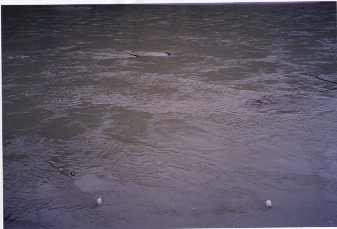
Fig. 3.14 a-d)- Time series of Type 2 boil diffusion (distance between markers= 8.7m)
