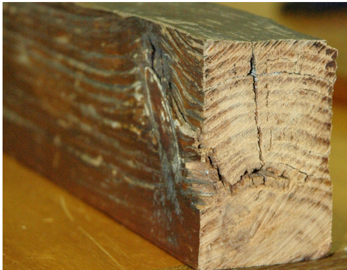
Figure 2.10: Image depicting the effect of brown rot in the middle of a surface coated pine board. The degradation is much different from that observed for normal weathering.
