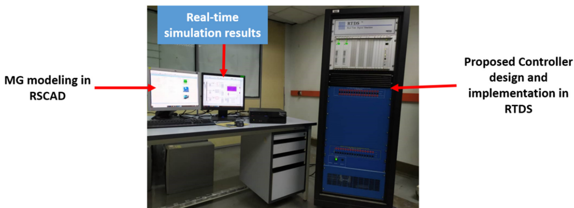
Figure 6. Laboratory setup of the proposed controller in AC MG with RTDS.
