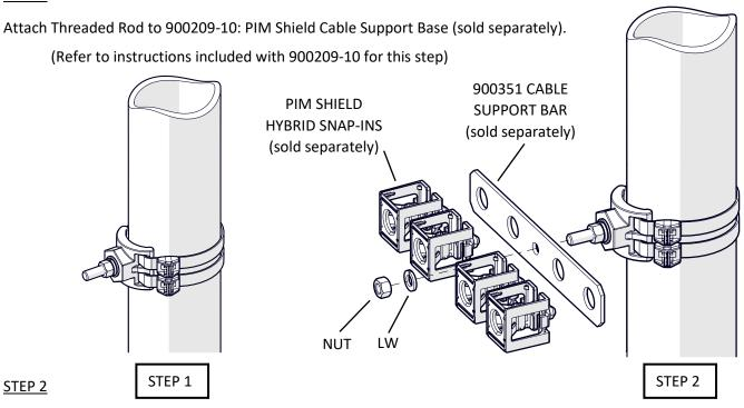
Install Cable Support Bar with hardware as shown (Torque hardware to 10 Ft-lb, ConcealFab Tool PN: 900053) (Note: Spare washers supplied with kit), then attach hybrid snap-in support(s) (sold-separately).
