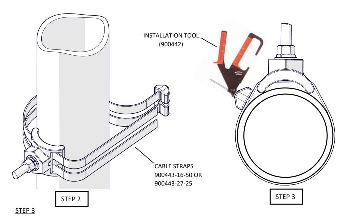
Use Cable Strap installation tool (900442 or equivalent) to tighten Cable Strap in position shown and flush-cut tail to Locking Head.
