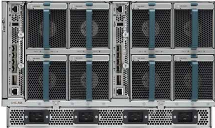
Figure 3 Cisco UCS 5108 Blade Server Chassis with 6324 Fabric Interconnects (rear view)
