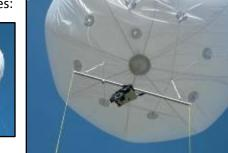
As airships become better-controlled and more stable, other sensors can be added to the payload. An airship could be used in tactical reconnaissance units to mount a small light-weight radar antenna, such as on the FARA-1E (Vol 1, pg 4-29). The Israeli Speed-A stabilized payload system with automated EO/thermal imager and laser rangefinder fits on lightweight airships.
