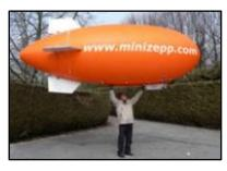
Mini-zepp blimps come in sizes 6-13 m, for use as aerostats or as dirigibles. The dirigibles include 2 electric motors and a gas-powered motor. Options include a video head and HF transmission system. In event of a power failure, a cable drops to the ground for recovery.
