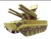
Pantsir-S1-0 System with Unified Turret on BMP-3 Chassis
