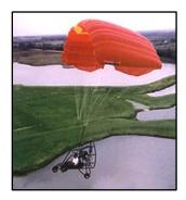
An efficient design for military units is to suspend a *trike* under the canopy and mount the paramotor onto it. Then the operator is freed to fly the craft; and can suspend combat gear to the frame. Some are erected at launch site, whereas others are solid welded structures. Trikes require larger parachutes
