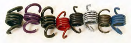
11. OLD STYLE NORAM SPRING $2.20 EACH HEAVY SHOE/LIGHT SHOE STALL SPEED BROWN (THIN) - 1620, 1800 RPM BLACK - 1900, 2100 RPM RED (STOCK, THIN) - 2040, 2500 RPM WHITE - 2470, 2900 RPM BLUE - 2650, 3200 RPM PURPLE - 2900, 3600 RPM GREEN - 3200, 4000 RPM ORANGE - 3500, 4400 RPM BROWN (THICK) - 3850, 4900 RPM $3.50 RED (THICK) - 4200, 5500 RPM $3.50
