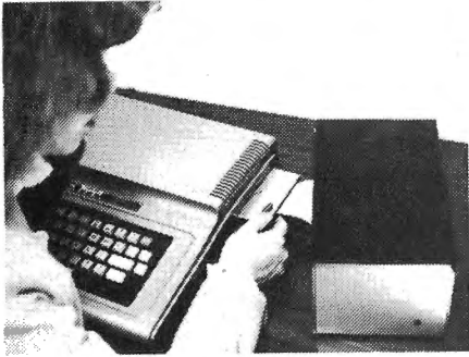
1. Here is Jeri plugging The Solution into the CoCo. Then she will move the main case up close to the CoCo. The cable is kept short to prevent noise and interference. The disk controller can be plugged into the side slot. The power supply plugs into a socket on the back of the case. All wires for the internal boards exit out the back of the case.
