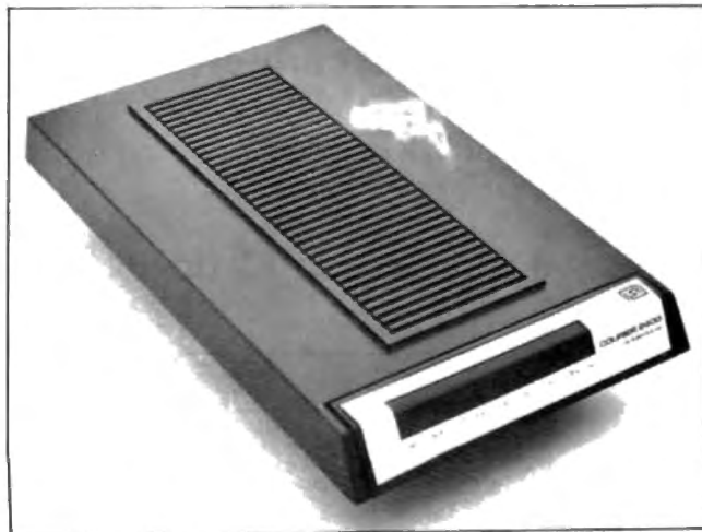
The Courier 2400 from U.S. Robotics uses advanced signal filtering technology for transmission at 2400 bits per second.
