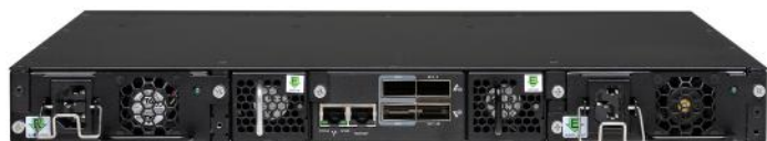
Figure 3: The Brocade ICX 6610 provides four 40 Gbps high-performance QSFP stacking ports (center) and dual, hot-swappable load-sharing power supplies and fan trays (left and right).
