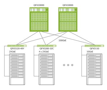
Figure 3. QFX5120-48Y in a leaf-and-spine deployment
