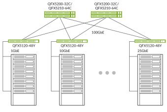
Figure 2. Edge-routed gateway at leaf with QFX5200/QFX5210 as spine
