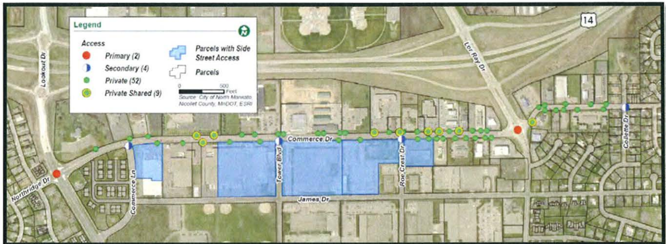
Figure 12. Access Points on Commerce Drive. Accesses in the eastern commercial business district are numerous contributing to driver confusion and pedestrian and bicycle safety issues.
