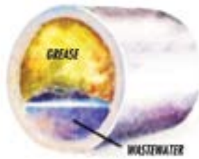
Sewer pipe clogged with grease
