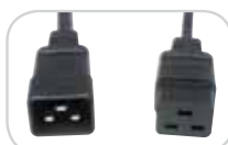
010-9342: C20 Male to C19 20A 8-foot, 12 AWG/3-wire
