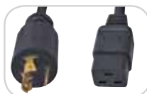
010-9339: L5-20P to C19 125V, 20A twist-lock 8-foot, 12 AWG/3-wire
