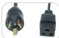
010-9341: L6-20P to C19 250V, 20A twist-lock 8-foot, 12 AWG/3-wire
