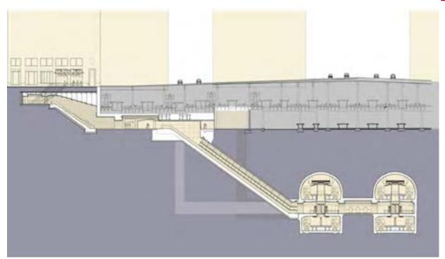
Cross section showing 8 new tracks and 4 platforms on 2 levels under existing Grand Central tracks
