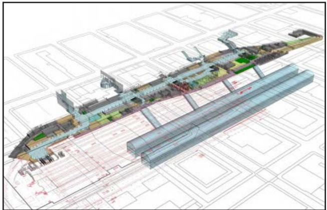
Isometric drawing of proposed new ESA station concourse and tunnels under Grand Central Terminal, highlighing four connecting escalator banks
