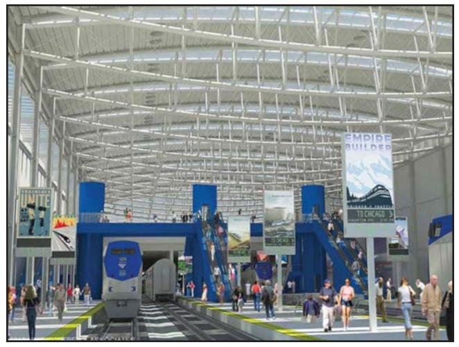
Rendering showing planned rehabilitated trainshed and new overhead walkways
