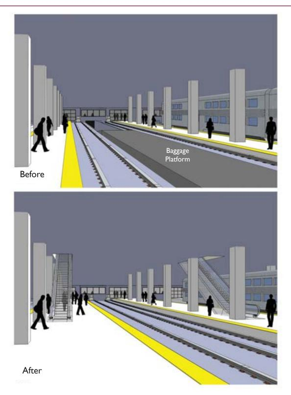
As shown in the BEFORE (top) and AFTER (bottom) images, eliminating unused baggage platforms would allow for passenger platforms to be widened and vertical circulation to be added.
