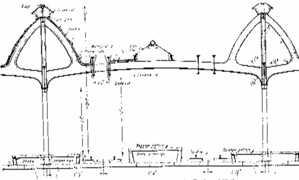
A Typical Cross Section of the Train Med, Station Tracks and Platforms
