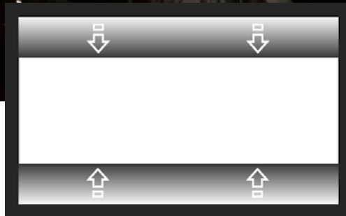
With two horizontal masks: The image base is constant and allows the projection of 3 formats.
