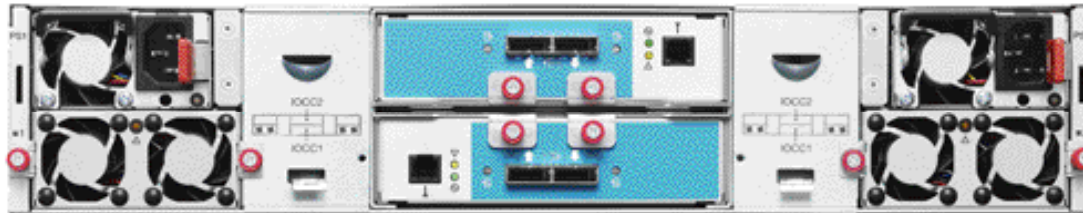
Rear View (With optional 2nd I/O module and 2nd power supply)
