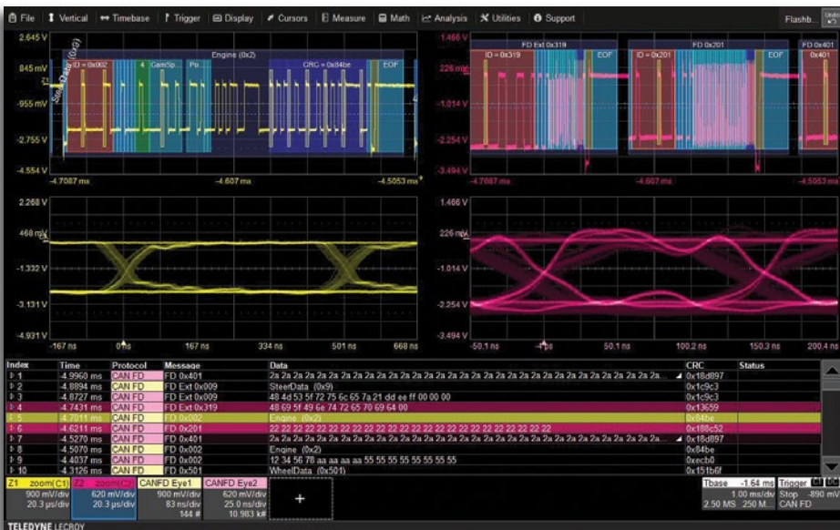
Eye diagrams “slice” each bit and overlay them to get a consolidated view of signal quality. Intrusions into the eye opening or onto a mask indicate potential problems.
