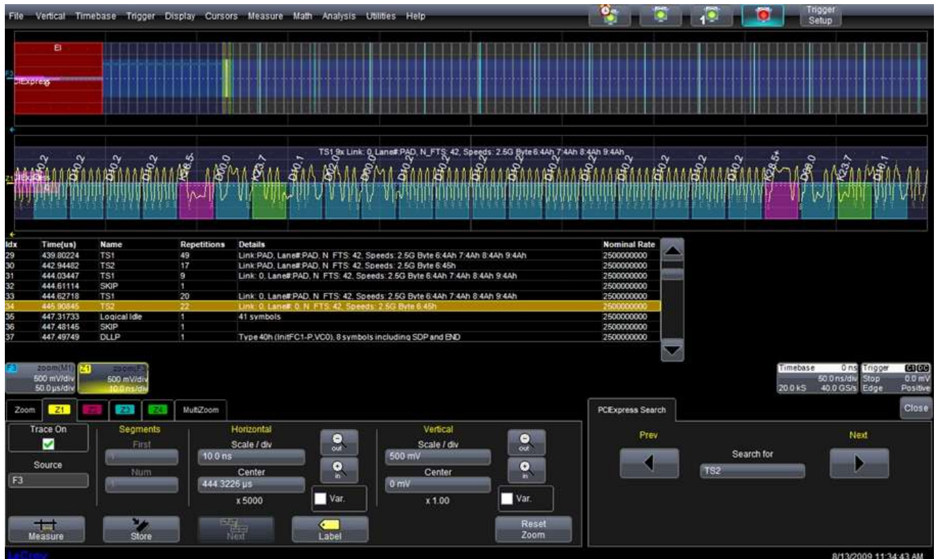
Zoomed in on Z1, showing the 8b/10b decode of a TS1 sequence.
