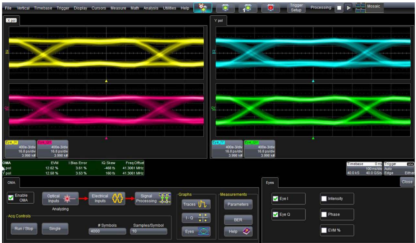
I and Q eye diagrams for a QPSK dual-Pol signal arranged in mosaic mode
