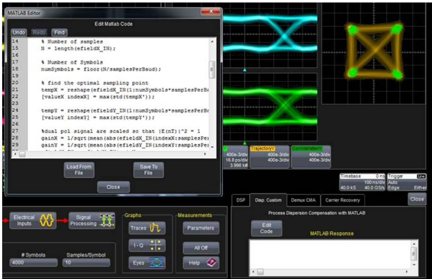
Custom scripts written in MATLAB™ can be called from within the OMA software
