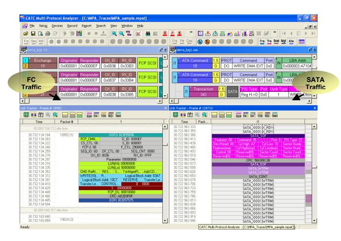
The Multiprotocol Analyzer provides a unified parent application in which CATC's SATracer and FCTracer can record and display traffic from two or more UPAS analyzers synchronized to single reference clock
