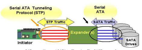
SATracer will record SATA traffic only – The SASTracer software option is required to capture SAS traffic including STP protocol
